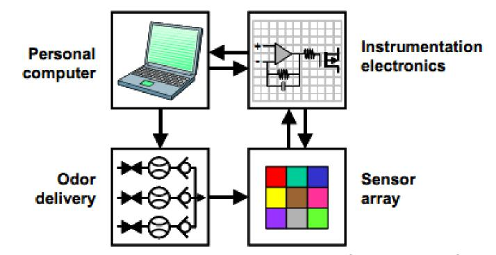
An electronic nose (e-nose) is a device that identifies the specific components of an odor and analyzes its chemical makeup to identify it. An electronic nose consists of a mechanism for chemical detection, such as an array of electronic sensors, and a mechanism for pattern recognition, such as a <u>neural network</u>
