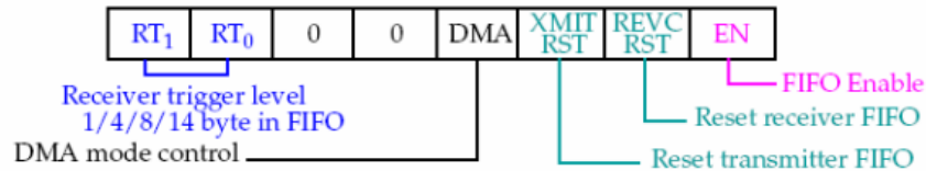
Figure 5 FIFO control register
