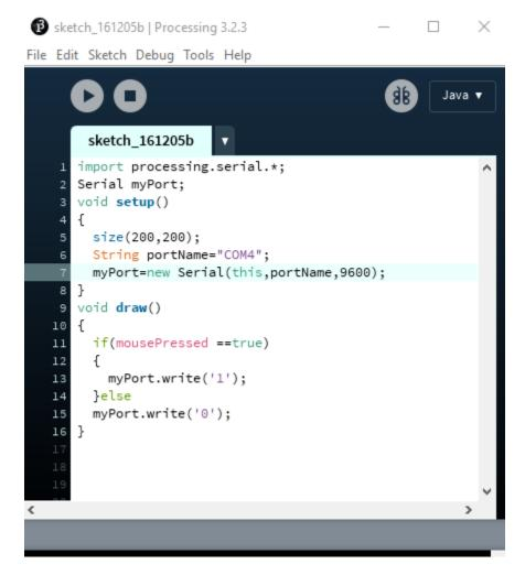
In our draw() loop, we send whatever we want over the serial port by using the write method from the Processing Serial library. For this sketch, we will send a '1' whenever we click our mouse in the Processing window. We'll also print it out on the console, just to see that we're actually sending something. If we aren't clicking we'll send a '0' instead.
