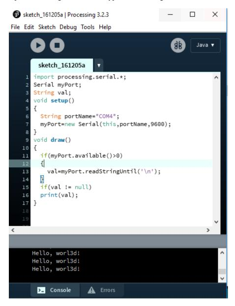
4- If you hit the 'run' button (and your Arduino is plugged in with the code on the previous page loaded up), you should see a little window pop-up, and after a sec you should see "Hello, World! "appear in the Processing console.
