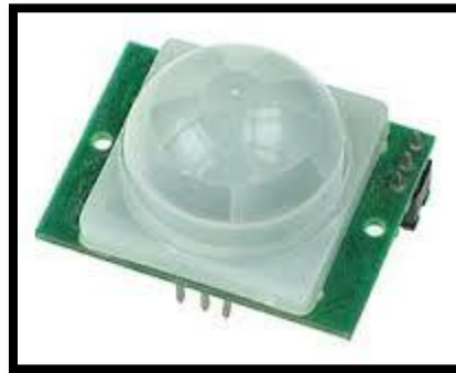
Fig. 4: PIR (motion detector) sensor
