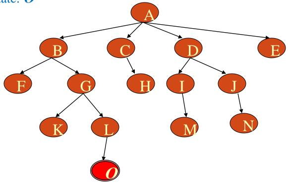
• The returned solution is the sequence of operators in the path:
