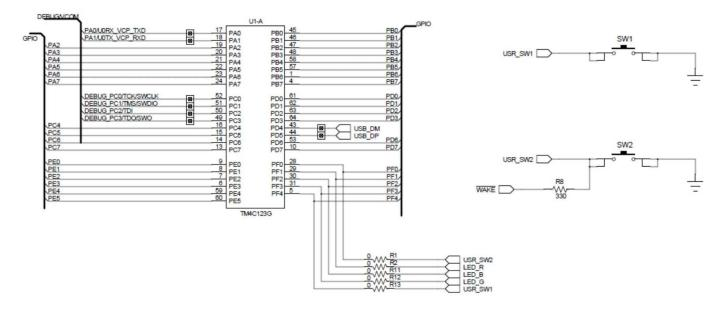
One end of both input switches is connected to the ground and the other end to PFO and PF4 pins. TM4C123GH6PM microcontroller provides internal pull-up resistors, which can be configured using GPIOPUR register. This line enables the pull-up resistor for PF4 and PFO pin.
