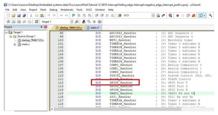
The linker script file will automatically replace the dummy implementation of GPIOF\_Handler inside the startup file with our defined implementation.
