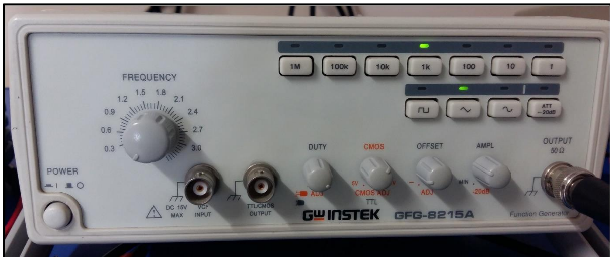
Figure 2.10: Function Wave Generator GFG-8215a
