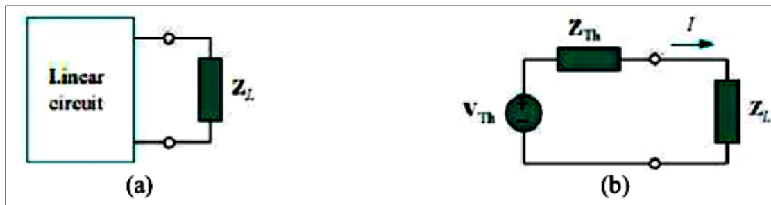
Figure 8.3: Finding maximum average power transfer: (a) circuit with a load, (b) Thevenin equivalent
