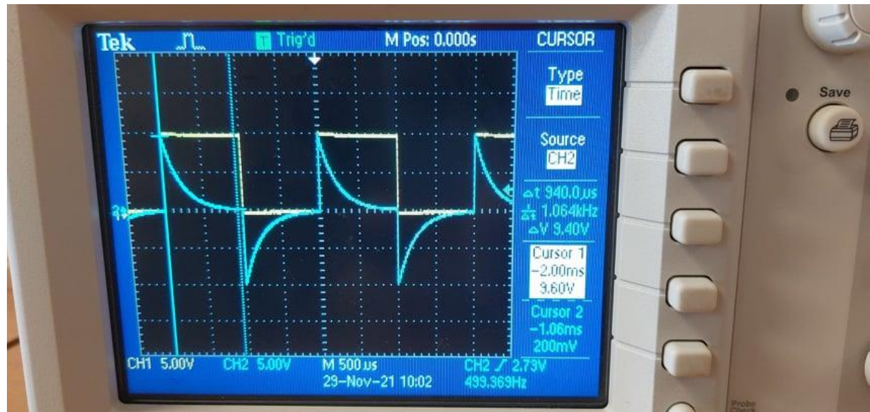
Figure 2. 5 RL circuit value of the measured steady state voltage
