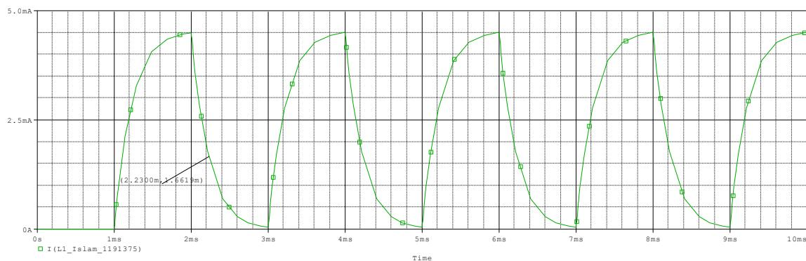
Time constant (at  $I = 1.666\text{mA}$ )  $\approx 2.23\text{mSec}$  (at 0.37 of  $I_p$  for discharging)
