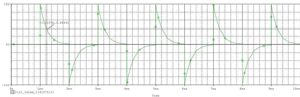
Time constant (at  $v = 3.6994V$ )  $\approx 1.2337\text{mSec}$  (at 0.37 of  $V_p$  for discharging)
