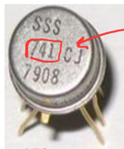
(c) TO-5 metal can 8-Leads package
