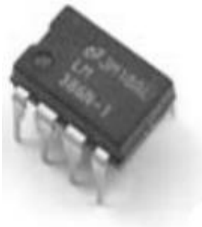
(a) Op Amp 741 8-pins DIP package
