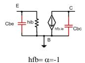
$$h_{fe}.i_b = h_{fe} \frac{v_{be}}{h_{ie}} = g_m v_{be};$$
