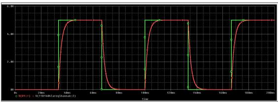
To be underdamped: a < w  $\rightarrow$  R / 2L < 1 /  $\vee$  (LC)  $\rightarrow$  R < 2L /  $\vee$  (LC)  $\rightarrow$  R < 4.47 K ohm
