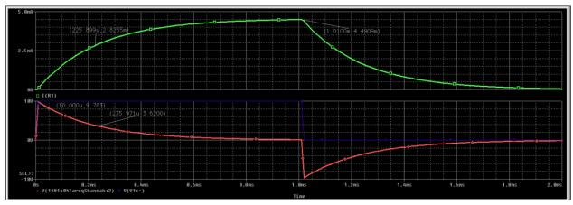
Since it's charging in the current response,  $I_{Charging} = 0.63 * 4.4909 mA = 2.829 m$ , t = T = 226 us Since it's discharging in the voltage response,  $V_{Discharging} = 0.37 * 9.783 = 3.62 v$ , t = T = 236 us t = T = L/R = 500 mH/2.2 k = 227 us (Theoretical)
