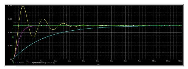
We can notice that when R=4.47k (Critical Damping – the pink curve), the output voltage is near from the input voltage (the green curve).
