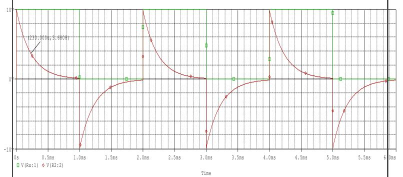
To calculate time constant, we use the assumption that it is at discharging when V(t) = 0.37 V max = 0.37\*10 = 3.7 volt
