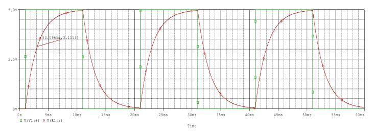
Steady state voltage value on the capacitor = 5 volt. To calculate time constant, we use the assumption that it is at charging when V(t) = 0.63\*V max = 0.63\*5 = 3.15v
