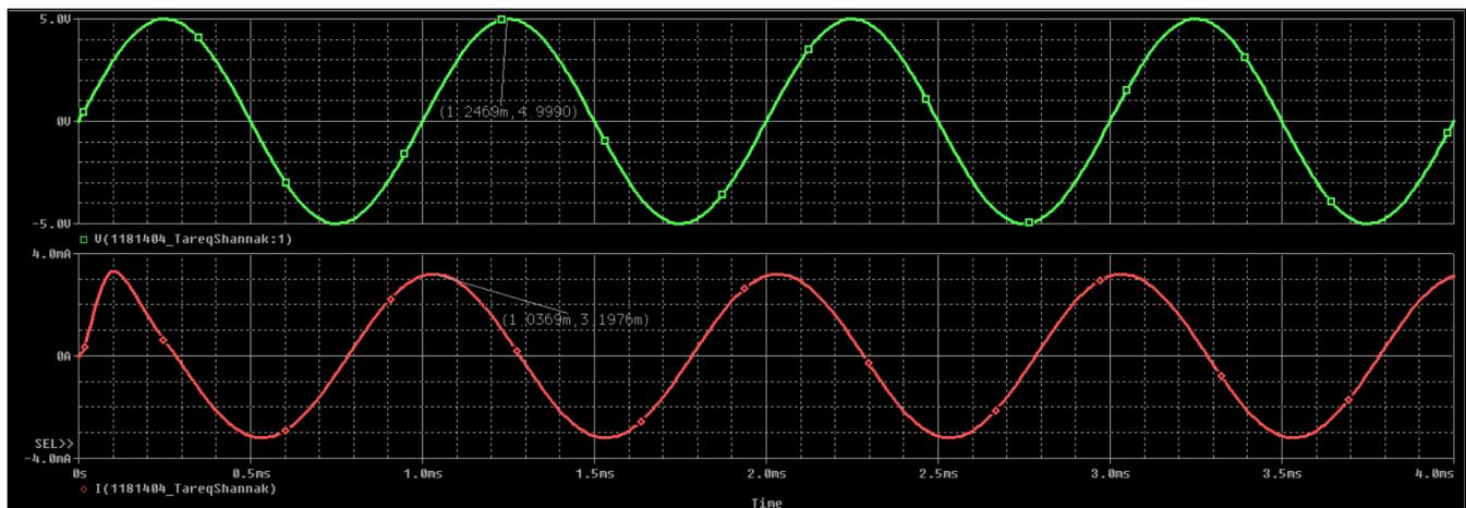
$$\text{From Graph: Phase Shift} = \frac{T_{\Delta pp} \times 360}{\text{Period}} = \frac{(1.0369\text{m} - 1.2469\text{m}) \times 360}{1\text{m}} = -75.6 \text{ degrees}$$
