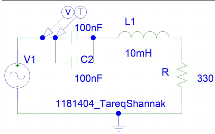
When we add a capacitor with value  $100\text{nF}$  in a parallel with the old one, the total capacitance =  $200\text{nF}$ .
