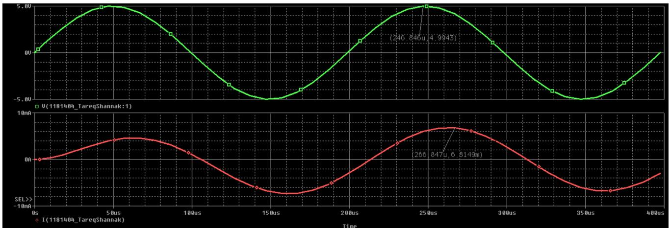
$$\text{From Graph: Phase Shift} = \frac{T_{\Delta pp} \times 360}{\text{Period}} = \frac{(266.847\mu - 246.846\mu) \times 360}{198.689\mu} = 36.24 \text{ degrees}$$
