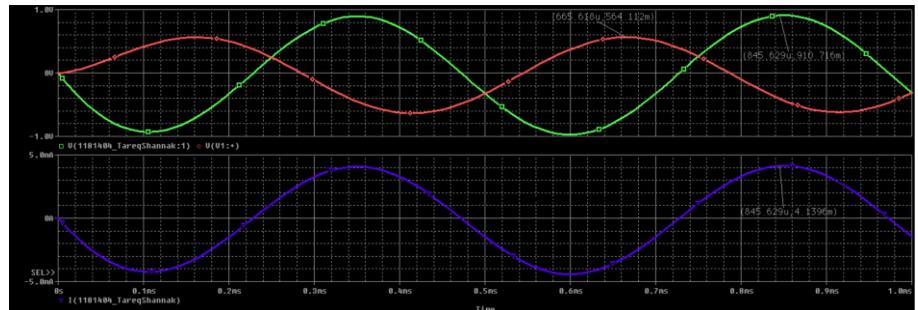
$$V_s = 564.112m, I_s = 4.1396mA, V_{220\Omega} = 910.716mv$$
