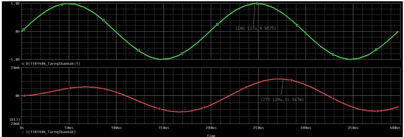
$$\text{From Graph: Phase Shift} = \frac{T_{\Delta pp} \times 360}{\text{Period}} = \frac{(276.129\mu - 246.127\mu) \times 360}{198.689\mu} = \mathbf{54.36 \text{ degrees}}$$
