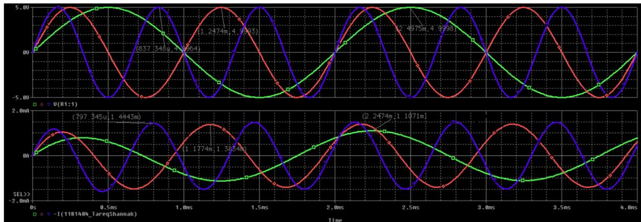
Because it's a capacitive circuit, current in all cases leads the voltage by a phase shift
