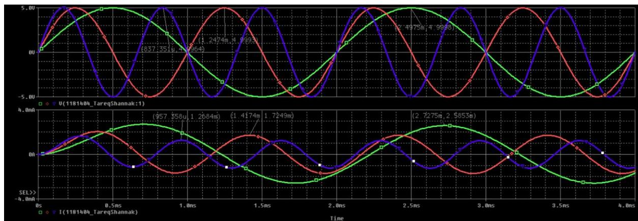
Because it's an inductive circuit, voltage in all cases leads the current by a phase shift
