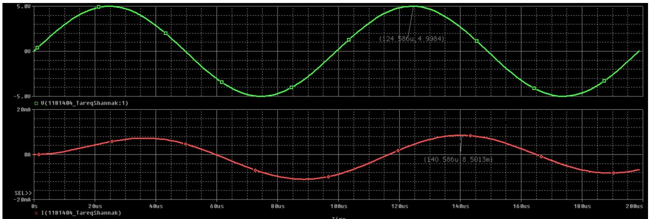
**From Graph:** Phase Shift =  $\frac{T_{app} \times 360}{Period} = \frac{(140.6\mu - 124.6\mu) \times 360}{99.344\mu} = 57.98 \text{ degrees}$
