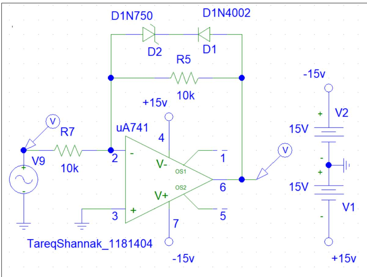
When the amplitude = 5V, there is a clipped output voltage
