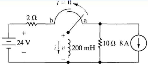
Assume that the switch in the circuit shown has been in position b for a long time, and at t = 0 it moves to position
