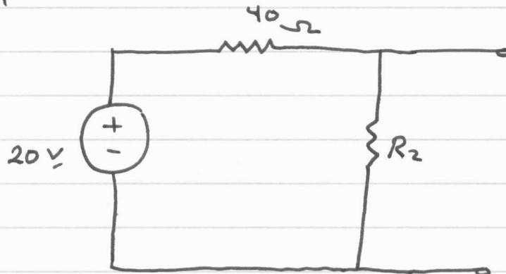
$$4 = \frac{R_2}{R_2+40} (20) \rightarrow R_2 = 10\Omega$$
