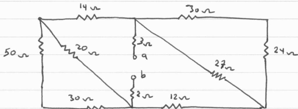
$$R_{\text{eq}} = 2 + 3 + \left[ \left( \left( 30 + 24 \right) \parallel 27 \right) + 12 \right] \parallel \left( 14 + (50 + 30) \parallel 20 \right)$$
