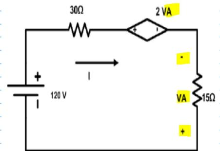
$$\begin{aligned} VA &= -I \times 15 \\ &= -120 \text{ V} \end{aligned}$$
