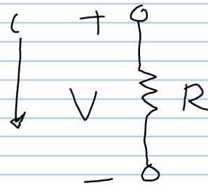
$$\begin{aligned} P &= V i \\ &= V \left( \frac{V}{R} \right) \\ \boxed{P} &= \frac{V^2}{R} \end{aligned}$$
