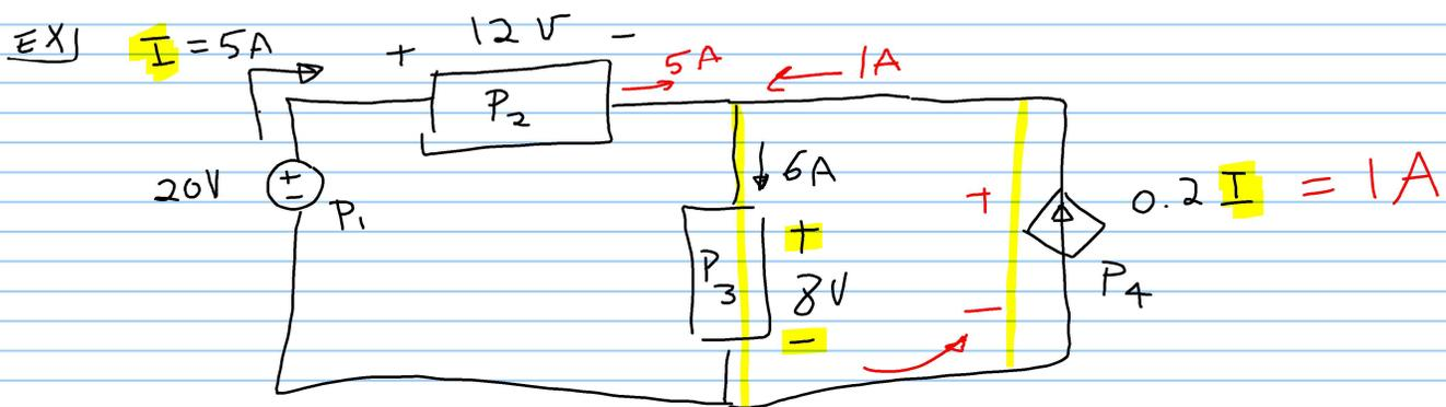
Calculate the power supplied or absorbed by each element
