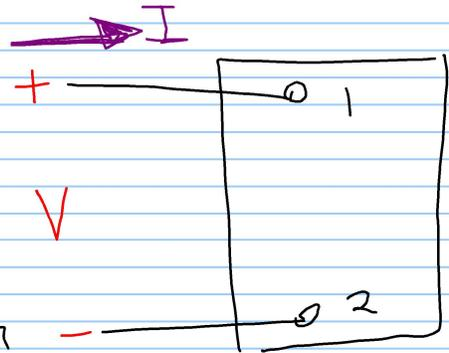
$$\boxed{P = VI} \quad \text{OR} \quad \boxed{P = -VI} \quad \text{Watts}$$
