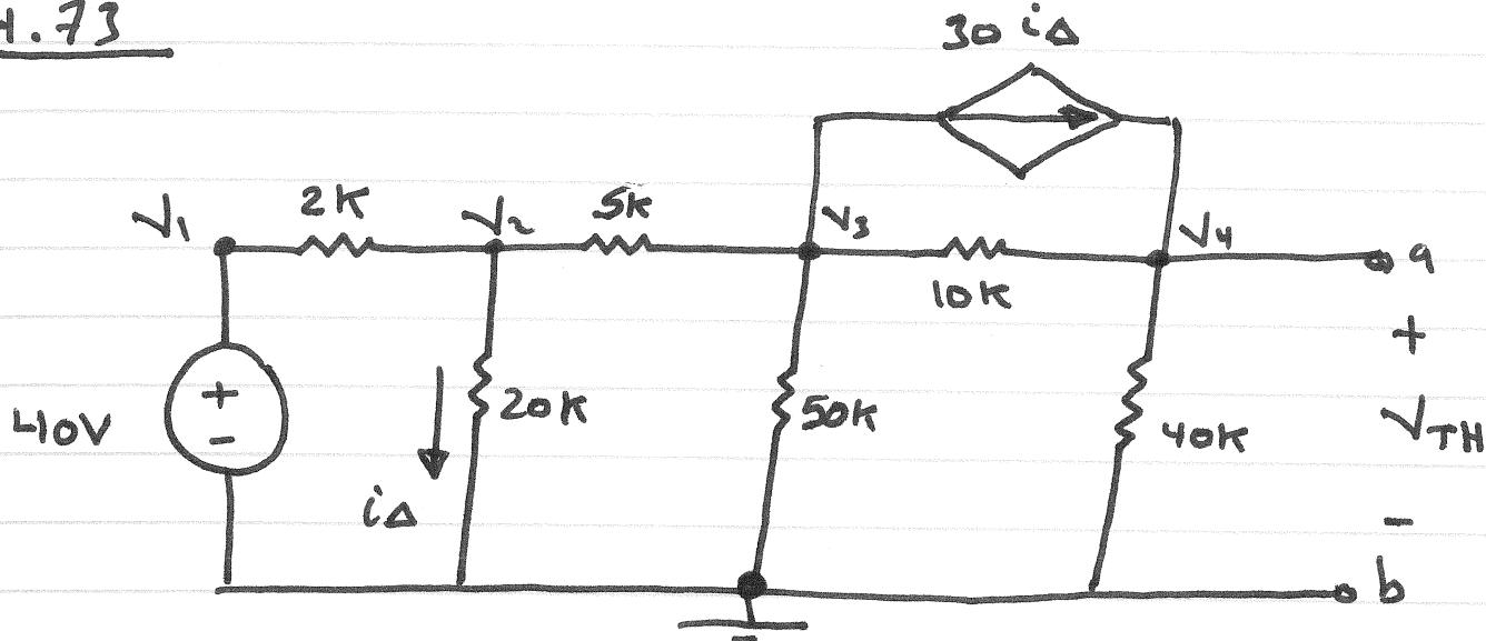
$$V_{TH} = V_4$$
