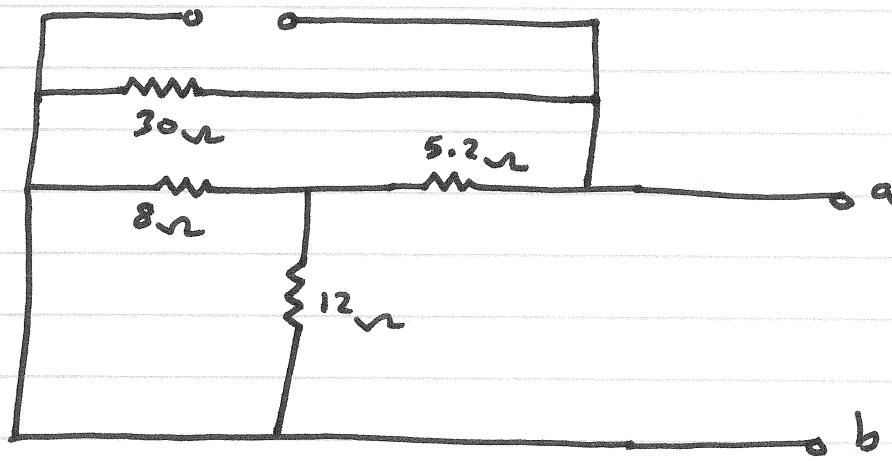
$$R_{TH} = 30\Omega \parallel (5.2\Omega + 8\Omega \parallel 12\Omega)$$
