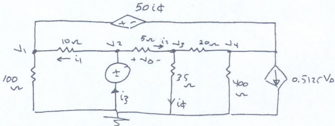
$$v_1 - v_4 = 50i\phi \quad ; \quad i\phi = \frac{v_2}{35}$$
