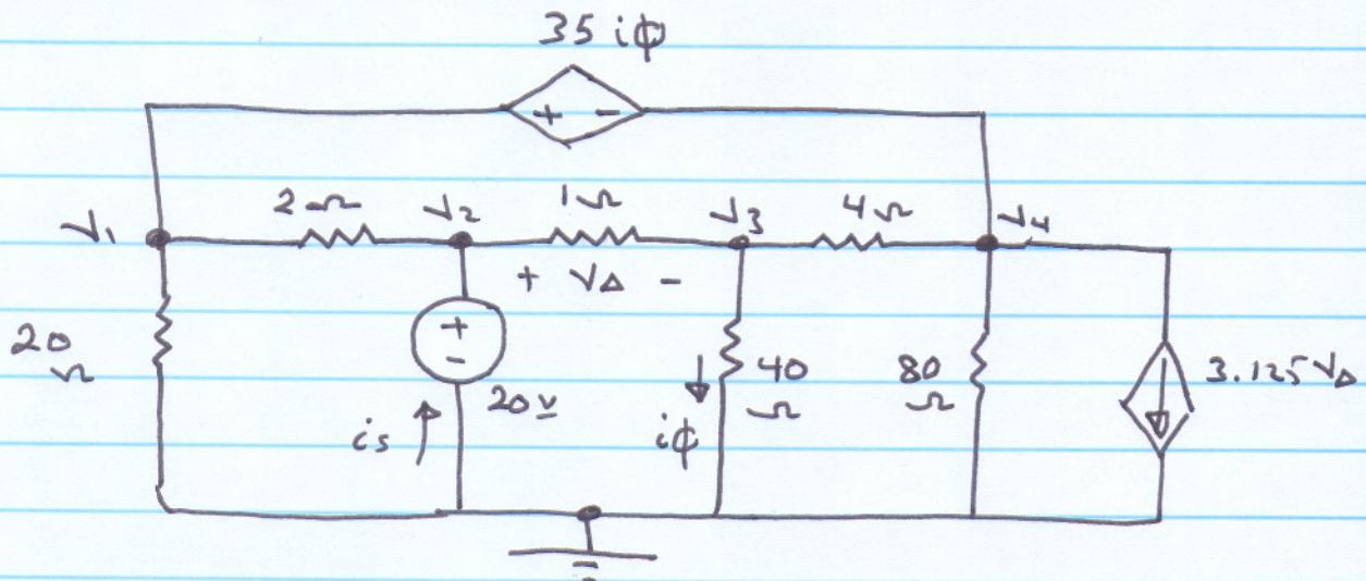
$$V_2 = 20 \text{ constrain equation}$$
