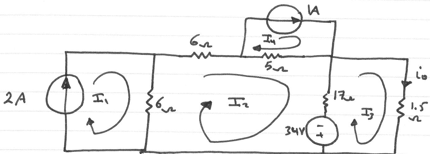
$$I_1 = 2A \quad \text{Constrain equation}$$
