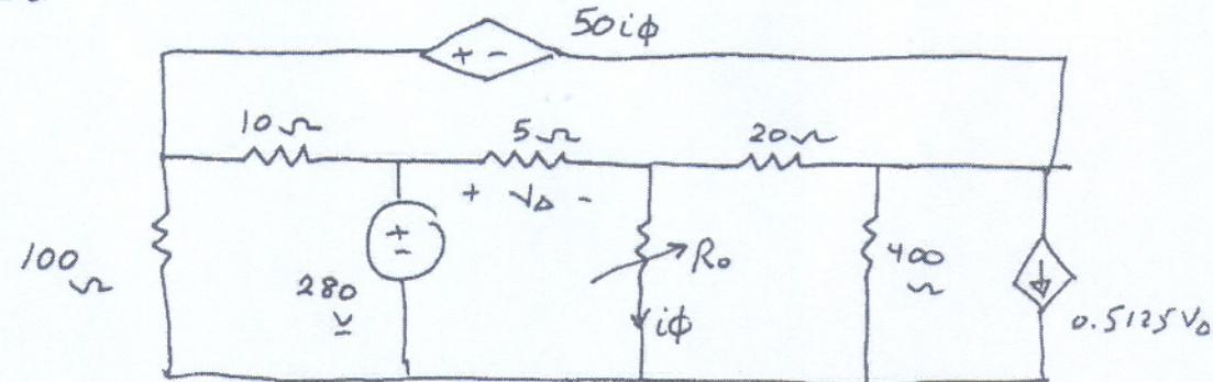
i) To find  $\text{V}_{TH}$ ;  $i\phi = 0 \rightarrow 50i\phi = 0 \rightarrow \text{Short Circuit}$
