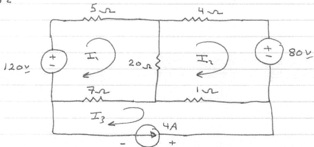
$$I_3 = -4A \quad \text{constraint equation}$$
