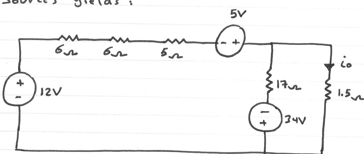
Combining the 12V and 5V into one source and adding the 3 resistors ( $6\Omega$ ,  $6\Omega$ , and  $5\Omega$ ) in series
