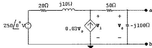
$$\frac{V_1 - 250}{20 + j10} - 0.03V_o + \frac{V_1}{50 - j100} = 0$$
