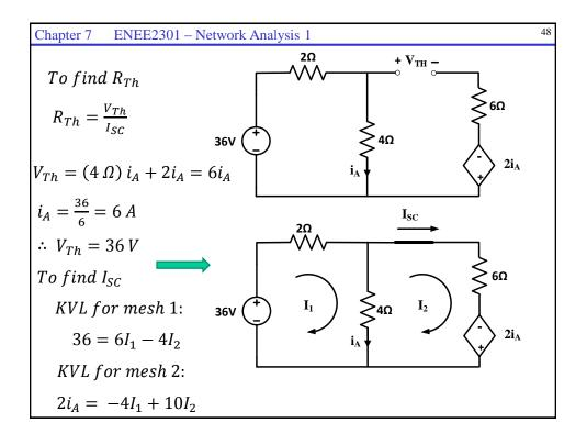
Chapter 7 ENEE2301 – Network Analysis 1  $i_A = I_2 - I_1$ Solving for  $I_2 = I_{SC} = \frac{36}{8} A$   $\therefore R_{Th} = \frac{V_{Th}}{I_{SC}} = 8 \Omega$   $\therefore \tau = \frac{L}{R_{Th}} = \frac{3}{8} s$   $\therefore v_0(t) = v_0(\infty) + [v_0(0^+) - v_0(\infty)] e^{-\frac{t}{\tau}} \qquad t > 0$   $\therefore v_0(t) = 27 + [18 - 27] e^{-\frac{t}{\tau}} \qquad t > 0$  $\therefore v_0(t) = (27 - 9 e^{-\frac{8}{3}t}) V \qquad for t > 0$
