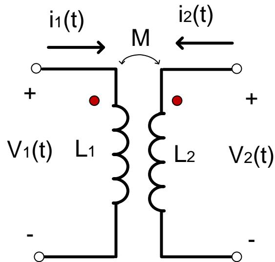
$$V_1(t) = L_1 \frac{d}{dt}(i_1(t)) + M \frac{d}{dt}(i_2(t))$$
