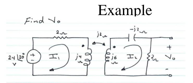
$24 \langle 30 = 2I_1 + j4I_1 - j2I_2 \rangle$  $24 \langle 30 = (2 + j4)I_1 - j2I_2 \dots (1)$
