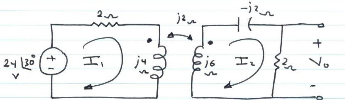
$$24 \angle 30^\circ = (2 + j4)I_1 - j2I_2 \dots\dots\dots(1)$$
