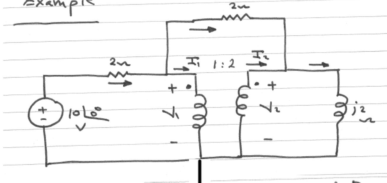
$$V_2 = 2V_1$$
