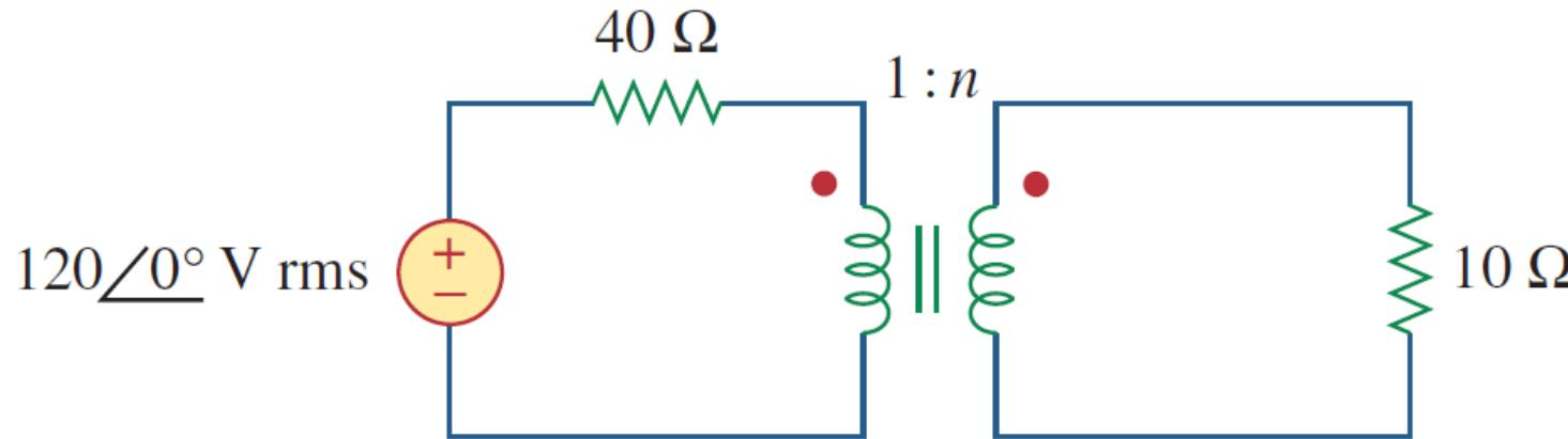
For maximum average power transfer to the load :  $Z_{th} = 10\Omega$
