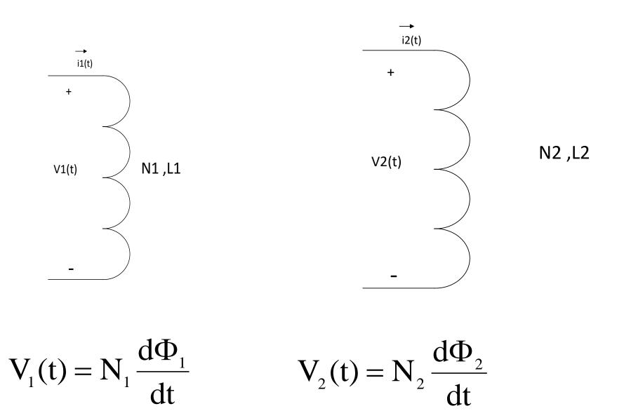
$$V_1(t) = N_1 \frac{d\Phi_1}{dt} \qquad \qquad V_2(t) = N_2 \frac{d\Phi_2}{dt}$$
