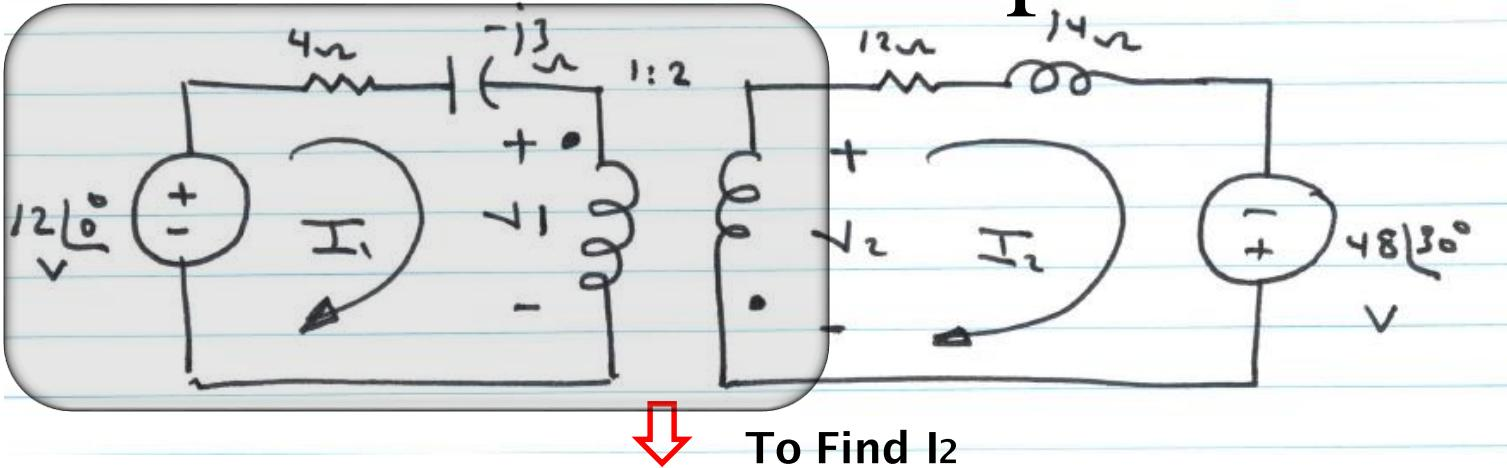
$$V_{TH1} = -nV_1 = -2(12 \angle 0^\circ) = -24 \angle 0^\circ$$
