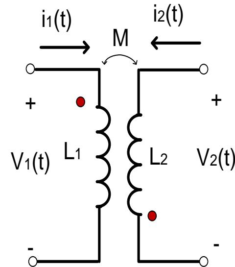
$$V_1(t) = L_1 \frac{d}{dt}(i_1(t)) + M \frac{d}{dt}(i_2(t))$$
