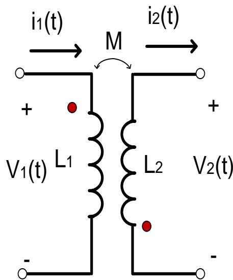
$$V_1(t) = L_1 \frac{d}{dt}(i_1(t)) + M \frac{d}{dt}(i_2(t))$$
