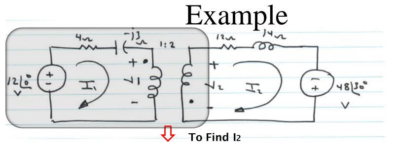
$$V_{\text{TH1}} = -nV_1 = -2(12 \ \langle 0^{\circ}) = -24 \ \langle 0^{\circ} \rangle$$
