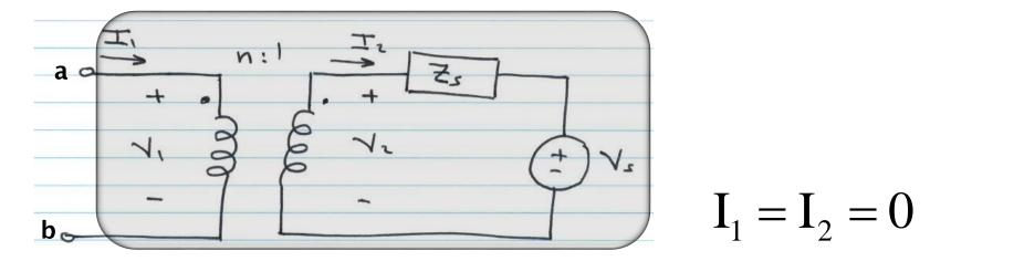
$V_{TH} = V_1 = nV_2 = nV_S$
