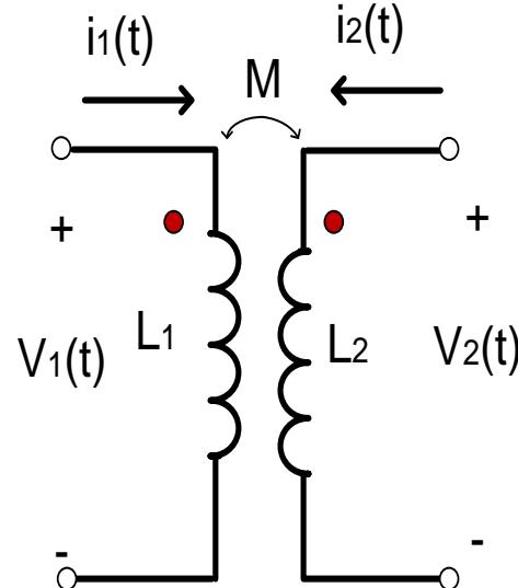
1-If both currents are directed into or away from **corresponding terminals**, the voltage due to the mutual inductance is of the same sign as the voltage due to self inductance
