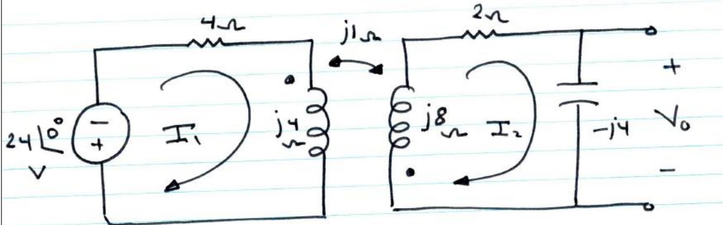
$$-24 \angle 0^\circ = (4 + j4)I_1 + j1I_2 \dots\dots\dots(1)$$
