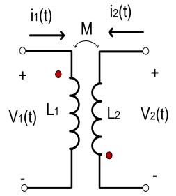
$$V_{1}(t) = L_{1} \frac{d}{dt} (i_{1}(t)) - M \frac{d}{dt} (i_{2}(t))$$
