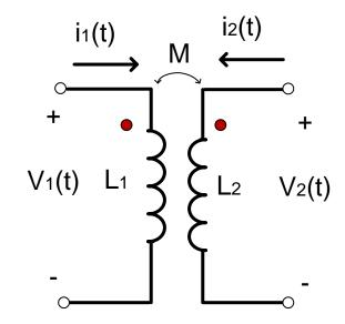
$$V_{1}(t) = L_{1} \frac{d}{dt} (i_{1}(t)) + M \frac{d}{dt} (i_{2}(t))$$
