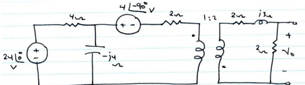
$$V_{TH1} = \frac{-j4}{4 - j4} 24 \angle 0^\circ - 4 \angle -90^\circ$$
