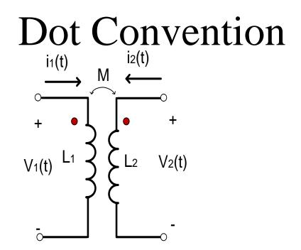
1-If both currents are directed into or away from corresponding terminals, the voltage due to the mutual inductance is of the same sign as the voltage due to self inductance
