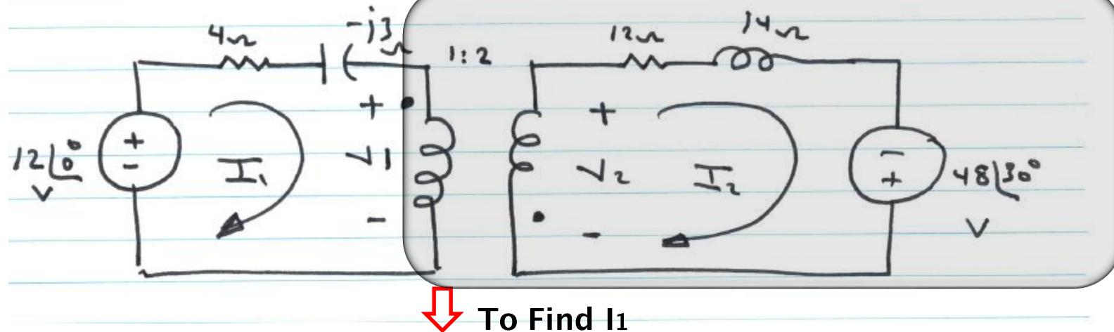
$$V_{TH2} = -\frac{1}{n}V_2 = -\frac{1}{2}(-48 \angle 30^\circ) = +24 \angle 30^\circ$$
