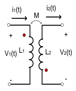
$$V_1(t) = L_1 \frac{d}{dt} (i_1(t)) + M \frac{d}{dt} (i_2(t))$$
