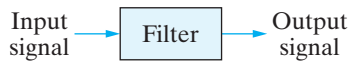
Figure 14.1 ▲ The action of a filter on an input signal results in an output signal.
