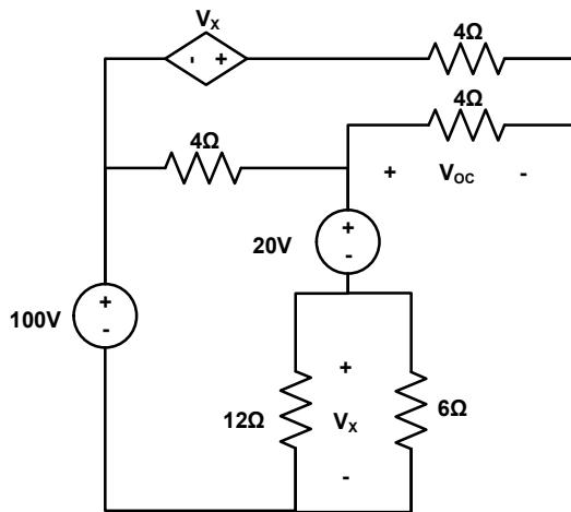
$$\frac{V_{oc}}{4} + \frac{V_x + 20 - 100}{4} + \frac{V_x}{4} + \frac{V_x + 20}{4} = 0$$
