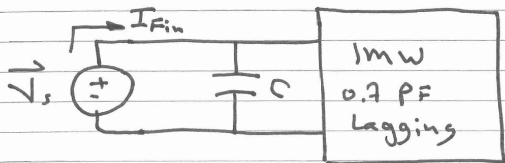
$$I_{Fin} = \frac{P_{av}}{(V_{rms})(PF_2)} = 483 \text{ A}_{rms}$$
