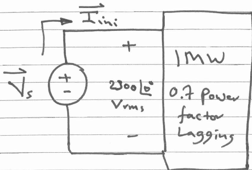
$$I_{ini} = \frac{P_{av}}{(V_{rms})(PF_1)} = 621 \text{ A}_{rms}$$
