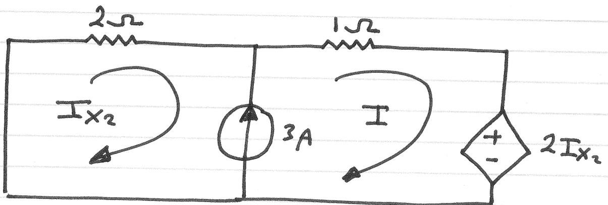
$$3 = I - I_{x2} \quad \text{Constraint equation}$$
