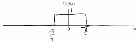
(ii) Assume that  $C(j\omega)$  is 1 for all  $\omega$  and  $x_c(t)$  is sufficiently band-limited so that the Nyquist criteria is met.  $x_c(t)$  consists of the superposition of s(t) which is the signal you are interested in and a 60Hz sinusoidal interference, i.e.,
