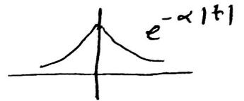
\* The FT of  $x(t)$  then is defined as the limit of the FT of  $y(t)$  as  $\alpha \rightarrow 0$
