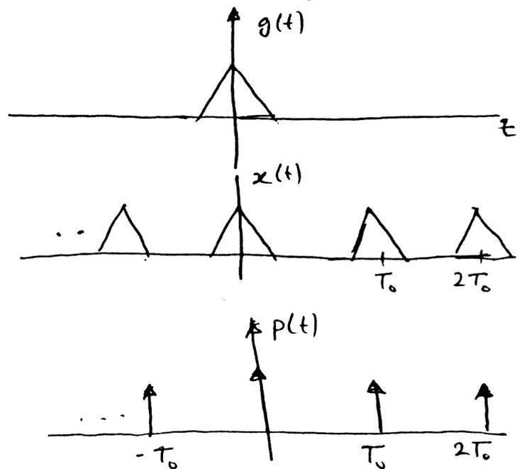
$p(t)$  is a periodic signal (train of impulses), hence using FS expansion :-
