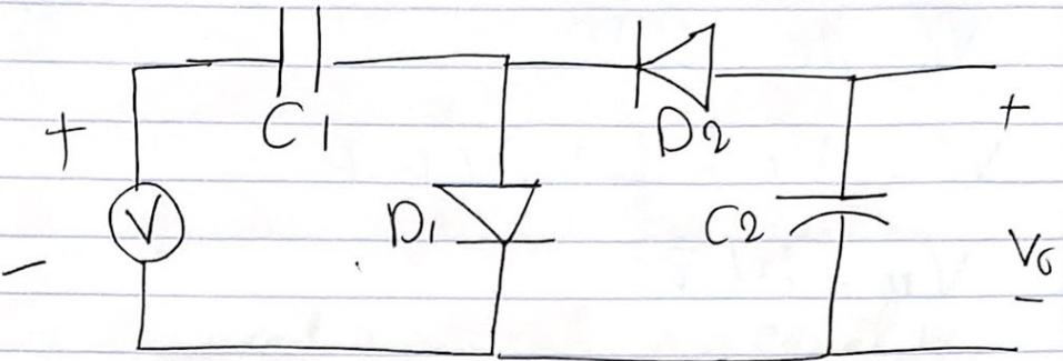
For the diode circuit shown, what will the output voltage  $V_o$  be in V if the input voltage  $V_i$  is a sine wave with an amplitude equal 6.4? Assume that when a diode is turned on the voltage across it will be 0.7V
