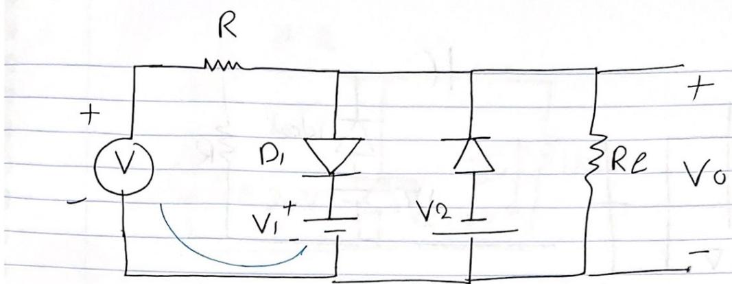
For the diode circuit shown, what will the output voltage,  $V_o$ , be in V if the input voltage  $V$  is equal to  $-10\text{V}$ ? Assume that when a diode is turned on the voltage across it will be  $0.7\text{V}$ , & for the batteries use  $V_1 = 5.1\text{V}$  &  $V_2 = 8.3\text{V}$ .  $R = 3.4\text{k}\Omega$ ,  $R_L = 19.6\text{k}\Omega$
