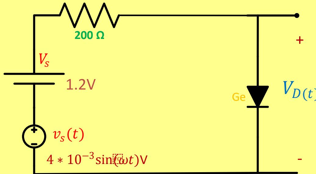
Since we have a dc source (1.2 V) and an ac signal ( $4 \times 10^{-3} \sin(\omega t)$  V) and the diode is always on ; we use superposition theorem to find  $V_D(t)$
