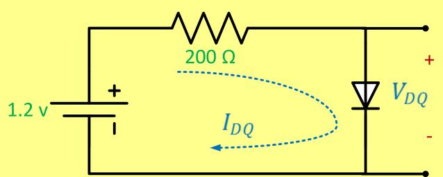
$$\therefore V_{DQ} = 0.3 \text{ v}$$
