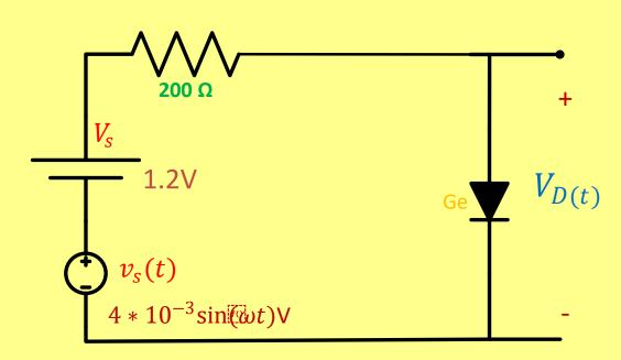
Since we have a dc source (1.2 V) and an ac signal  $(4x10^{-3} \sin \omega t \text{ V})$  and the diode is always on; we use superposition theorem to find  $V_D(t)$
