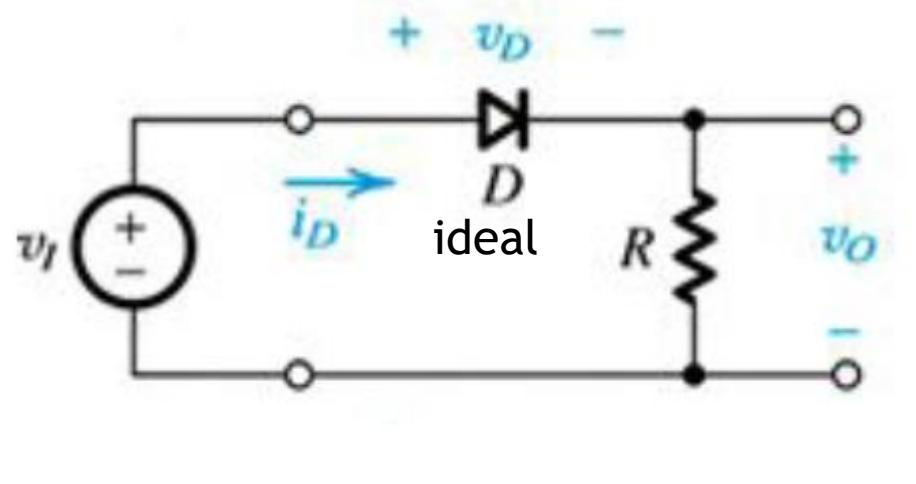
**A) when  $V_i(t) > 0$ , Diode is on (short circuit)**
