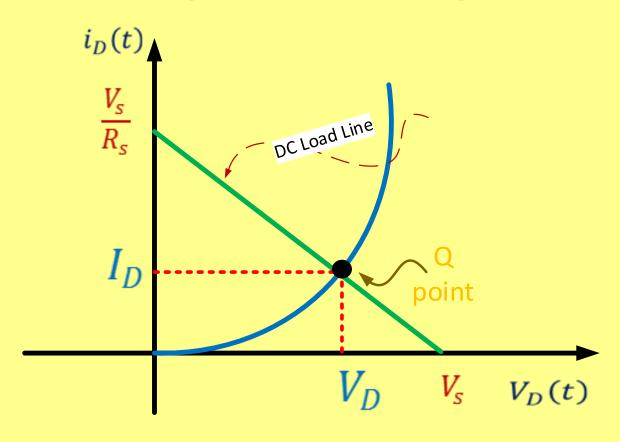
$$I_D = - \frac{1}{R_S} V_D + \frac{V_S}{R_S}$$
