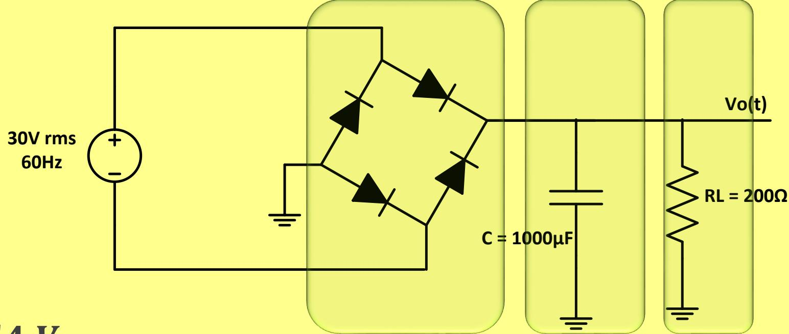
►  $V_{L,dc} = V_m - \frac{V_m}{4f_o R_L C} = 41.54 \text{ V}$
