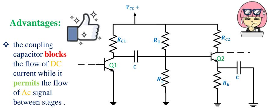
❖ It makes it possible to have a dc bias voltage at the output of one stage that is different from the dc bias voltage at the input to the next stage (stage isolation)
