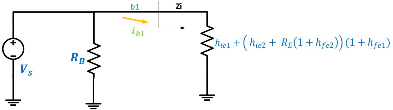
$$Z_i = h_{ie1} + (h_{ie2} + R_E (1+h_{fe2})) (1+h_{fe1})$$
