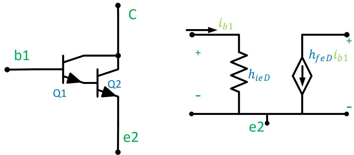
$$\therefore h_{ieD} = h_{ie1} + \frac{(1+h_{fe1})V_T}{I_{E1}}$$
