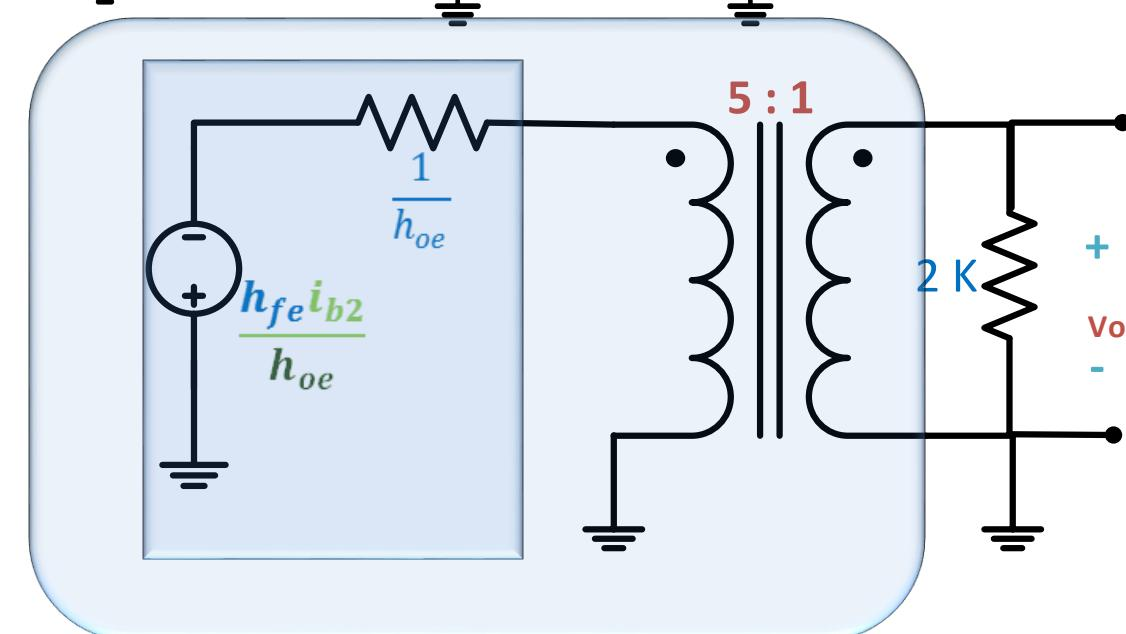
$$V_o = -\frac{2K}{2K+2K} \frac{h_{fe} i_{b2}}{5h_{oe}}$$
