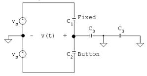
$$C_1 \frac{d(v - v_s)}{dt} + C_2 \frac{d(v + v_s)}{dt} + C_3 \frac{dv}{dt} = 0$$
