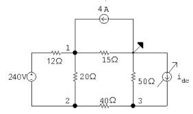
Since the 4 A source is developing 0 W,  $v_1$  must be 0 V.
