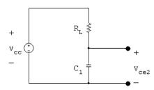
It follows that  $v_{\text{ce}2} = V_{CC} - V_{CC}e^{-t/R_{\text{L}}C_1}$ .
