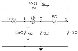
$$\frac{v_2}{5} + 2 + \frac{v_2 - v_3}{5} = 0$$
