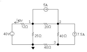
$$\frac{v_1 + 40}{12} + \frac{v_1}{25} + \frac{v_1 - v_2}{20} + 5 = 0$$
