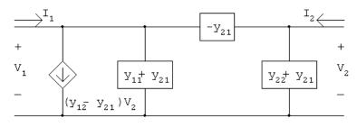
$$I_1 = y_{11}V_1 + y_{12}V_2;$$
