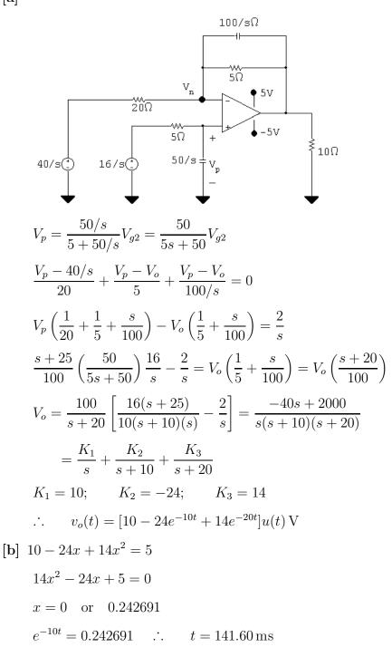
P 13.48 Let  $v_{o1}$  equal the output voltage of the first op amp. Then
