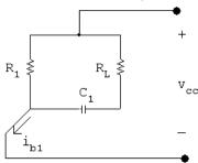
$$i_{b1} = \frac{V_{CC}}{R_1} + \frac{V_{CC}}{R_L} e^{-t/R_L C_1}$$
