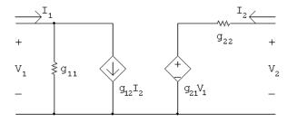
[b] The g parameters for the first two port in Fig P 18.38(a) are
