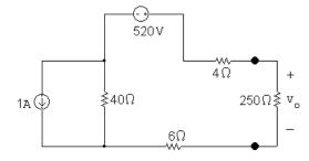
Next use a source transformation to convert the 1 A current source and  $40\,\Omega$  resistor:
