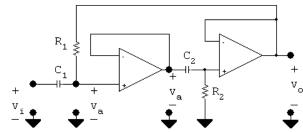
At low frequencies the capacitors appear as open circuits and hence the output voltage is zero. As the frequency increases the capacitor branches approach short circuits and  $v_a = v_i = v_o$ . Thus the circuit is a unity-gain, high-pass filter.
