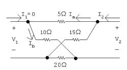
$$V_1 = V_a - V_b; \quad V_a = \frac{10}{15} V_2; \quad V_b = \frac{20}{35} V_2$$
