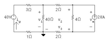
$$\frac{v_1}{40} + \frac{v_1 - 40}{4} + \frac{v_1 - v_2}{2} = 0 \quad \text{so} \quad 31v_1 - 20v_2 + 0v_3 = 400$$
