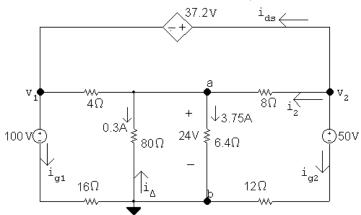
Using the node voltage method to find  $v_1$  and  $v_2$  yields
