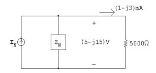
$$I_N = \frac{5 - j15}{Z_N} + (1 - j3) \,\text{mA}, \quad Z_N \text{ in } k\Omega$$
