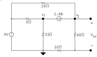
$$\frac{v_2 - 9}{20} + \frac{v_2}{70} - 1.8 = 0$$
