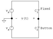
$$C_1 \frac{d}{dt}(v - v_s) + C_2 \frac{d}{dt}(v + v_s) = 0$$
