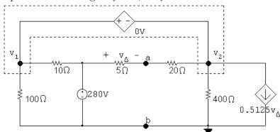
$$\frac{v_1}{100} + \frac{v_1 - 280}{10} + \frac{v_1 - 280}{25} + \frac{v_1}{400} + 0.5125v_{\Delta} = 0$$
