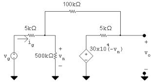
Write the node voltage equation at the left hand node:
