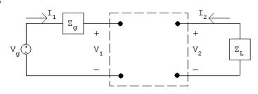
$$V_2 = b_{11}V_1 - b_{12}I_1; \qquad V_1 = V_g - I_1Z_g$$
