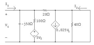
$$I_1 = \frac{V_1}{-i50} + \frac{V_1}{100} + \frac{V_1}{20} = V_1 \frac{(6+i2)}{100}$$
