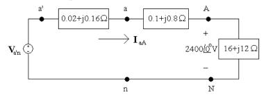
[a] We can find the line current using Ohm's law, since the a-phase line current is the current in the a-phase load. Then we can use the fact that  $\mathbf{I}_{aA}$ ,  $\mathbf{I}_{bB}$ , and  $\mathbf{I}_{cC}$  form a balanced set to find the remaining line currents. Note that since we were not given any phase angles in the problem statement, we can assume that the phase voltage given,  $\mathbf{V}_{AN}$ , has a phase angle of  $0^{\circ}$ .
