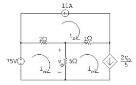
There are current sources on the perimeters of both the  $i_b$  mesh and the  $i_c$  mesh, so we know that
