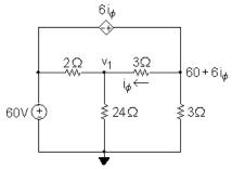
The node voltage equation at  $v_1$  is
