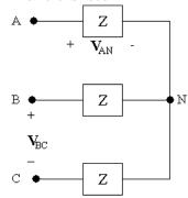
We know  $V_{AN}$  and wish to find  $V_{BC}$ . To do this, write a KVL equation to find  $V_{AB}$ , and use the known phase angle relationship between  $V_{AB}$  and  $V_{BC}$  to find  $V_{BC}$ .
