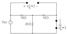
$$v_o(\infty) = 75 \text{ V}; \qquad i_o(\infty) = \frac{75}{10 + (200/30)} \cdot \frac{20}{30} = 3 \text{ A} \quad \text{Checks}$$
