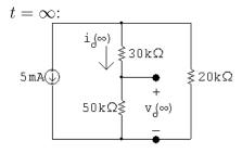
$$i_o(\infty) = -5 \times 10^{-3} \left(\frac{20}{100}\right) = -1 \,\text{mA}; \qquad v_o(\infty) = i_o(\infty)(50,000) = -50 \,\text{V}$$
