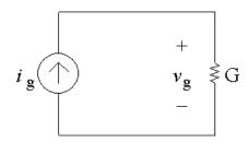
[a] Note from the circuit that the current through the conductance G is  $i_g$ , flowing from top to bottom, because the current source and the conductance are in the same branch of the circuit so must have the same
