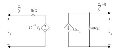
$$V_1 = 10^3 I_1 + 10^{-4} V_2 = 10^3 (-0.5 \times 10^{-6}) V_2 + 10^{-4} V_2$$
