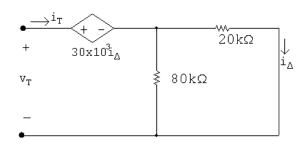
$$v_T = 30 \times 10^3 i_\Delta + 16 \times 10^3 i_T = 30 \times 10^3 (0.8) i_T + 16 \times 10^3 i_T = 40 \times 10^3 i_T$$
