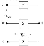
We know  $V_{CN}$  and wish to find  $V_{AB}$ . To do this, write a KVL equation to find  $V_{BC}$ , and use the known phase angle relationship between  $V_{AB}$  and  $V_{BC}$  to find  $V_{AB}$ .
