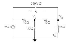
$$\frac{V_1 - 75/s}{10} + \frac{V_1}{20} + \frac{V_1 - V_2}{10} = 0$$
