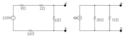
Finally, combine the  $20\,\Omega$  and  $12\,\Omega$  parallel resistors to give  $R_{\rm N} = 20 \| 12 = 7.5\,\Omega$ . Thus, the Norton equivalent circuit is the parallel combination of a 6 A source and a 7.5  $\Omega$  resistor.
