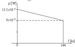
Note that in constructing the plot above, we used the fact that 40 hr  $= 144{,}000 \text{ s} = 144 \text{ ks}$
