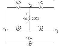
$$\frac{v_1 - v_2}{5} + \frac{v_1}{7} - 16 = 0$$
