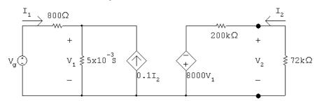
$$V_2 = \frac{-8000V_1(72)}{272}$$
