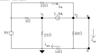
$$\frac{v_2 - 9}{20} + \frac{v_2}{10} - 1.8 = 0$$
