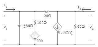
$$\frac{V_2 - V_1}{20} + 0.025V_1 + \frac{V_2}{40} = 0$$
