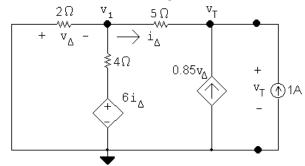
$$\frac{v_1}{2} + \frac{v_1 - 6i_{\Delta}}{4} + \frac{v_1 - v_T}{5} = 0$$
