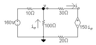
$$\frac{v_o - 160}{10} + \frac{v_o}{100} + \frac{v_o - 150i_\sigma}{50} = 0; \quad i_\sigma = -\frac{v_o}{100}$$
