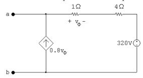
$$\frac{V_{\rm Th} - 320}{5} - 0.8 \left(\frac{V_{\rm Th} - 320}{5}\right) = 0 \qquad V_{\rm Th} = 320 \,\text{V}$$
