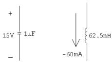
$$i_R(0) = \frac{15}{100} = 150 \,\text{mA}; \qquad i_L(0) = -60 \,\text{mA}$$
