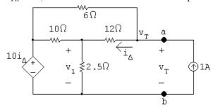
$$\frac{v_1 - 10i_{\Delta}}{10} + \frac{v_1}{2.5} + \frac{v_1 - v_{\mathrm{T}}}{12} = 0$$
