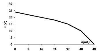
[b] Since the plot is linear for  $0 \le i_s \le 24$  mA amd since  $R = \Delta v/\Delta i$ , we can calculate R from the plotted values as follows:
