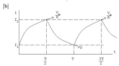
The steady-state current will alternate between  $I_1$  and  $I_2$  in exponential traces as shown. Assuming t = 0 at the instant i increases toward  $(V_m/R)$ , we have
