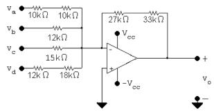
P 5.14 [a] Write a KCL equation at the inverting input to the op amp:
