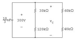
$$R_e = 150||100 = 60 \text{ k}\Omega; \qquad \tau = \left(\frac{10}{3} \times 10^{-9}\right) (60,000) = 200 \,\mu\text{s}$$
