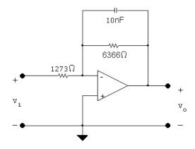
[b] Both the cutoff frequency and the passband gain are changed.
