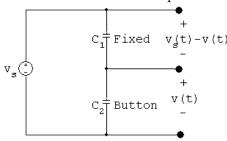
$$C_2 \frac{dv}{dt} = C_1 \frac{d}{dt} (v_s - v)$$
