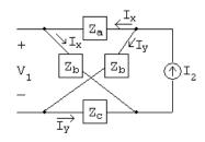
$$V_1 = Z_b I_x - Z_c I_y = Z_b I_x - Z_c (I_2 - I_x) = (Z_b + Z_c) I_x - Z_c I_2$$
