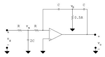
$$2C\frac{dv_{a}}{dt} + \frac{v_{a} - v_{g}}{R} + \frac{v_{a}}{R} = 0$$
