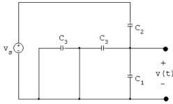
$$C_1 \frac{dv}{dt} + C_3 \frac{dv}{dt} + C_2 \frac{d(v - v_s)}{dt} = 0$$
