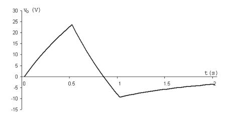
[d] No, the circuit has memory because of the capacitive storage element.
