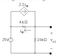
$$\frac{v_{o1} - 25}{4000} + \frac{v_{o1}}{20,000} - 2.2\left(\frac{v_{o1} - 25}{4000}\right) = 0$$
