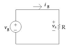
[a] The resistor and the voltage source are in parallel and the resistor voltage and the voltage source have the same polarities. Therefore these two voltages are the same:
