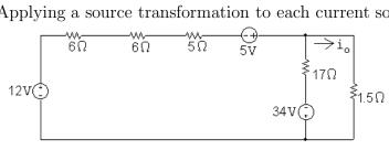
Now combine the 12 V and 5 V sources into a single voltage source and the 6  $\Omega$ , 6  $\Omega$  and 5  $\Omega$  resistors into a single resistor to get
