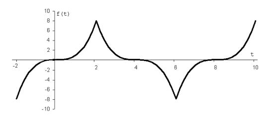
[c] f(t) has quarter-wave symmetry, since f(T/2 - t) = f(t) in the interval 0 < t < 4.
