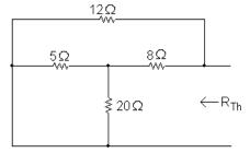
Note that the  $5\Omega$  and  $20\Omega$  resistors are in parallel, with an equivalent resistance of  $5\|20 = 4\Omega$ . The equivalent  $4\Omega$  resistance is in series with the  $8\Omega$  resistor for an equivalent resistance of  $4 + 8 = 12\Omega$ . Finally, the  $12\Omega$  equivalent resistance is in parallel with the  $12\Omega$  resistor, so  $R_{\rm Th} = 12\|12 = 6\Omega$ .
