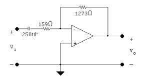
[b] The passband gain changes but the cutoff frequency is unchanged.
