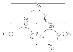
The 2 A current source is shared by the meshes  $i_a$  and  $i_b$ . Thus we combine these meshes to form a supermesh and write the following equation:
