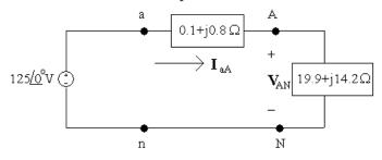
[a] Find the a-phase line current from the a-phase circuit:
