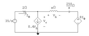
$$\frac{V_o - 35/s}{2} + 0.4V_\Delta + \frac{V_o - 8I_\phi}{s + (250/s)} = 0$$
