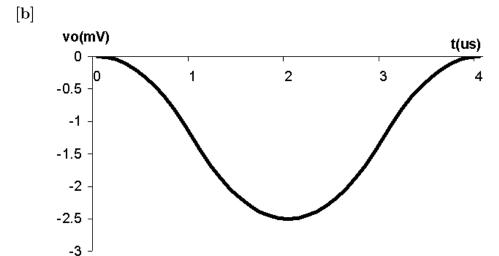
[c] The output voltage will also repeat. This follows from the observation that at  $t=4\,\mu s$  the output voltage is zero, hence there is no energy stored in the capacitor. This means the circuit is in the same state at  $t=4\,\mu s$  as it was at t=0, thus as  $v_g$  repeats itself, so will  $v_o$ .
