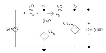
$$\frac{v_1 - 24}{2} + \frac{v_1 - 6i_{\Delta}}{4} + \frac{v_1 - 42}{5} = 0$$
