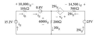
[a] To find  $i_{\beta}$ , write a KVL equation around the left-hand loop, summing voltages in a clockwise direction starting below the 15.2V source:
