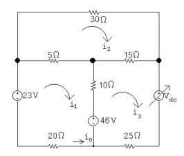
Write the mesh current equations. Note that if  $i_o = 0$ , then  $i_1 = 0$ :
