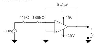
$$v_o = -\frac{1}{RC_f} \int_0^{32 \times 10^{-3}} -10 \, dt + 0 = -\frac{1}{RC_f} (-10t) \Big|_0^{32 \times 10^{-3}} = -\frac{1}{RC_f} (-320 \times 10^{-3})$$
