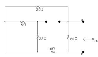
$$R_{\rm Th} = (20 + 10 || 60 = 20 \Omega \text{ (CHECKS)})$$
