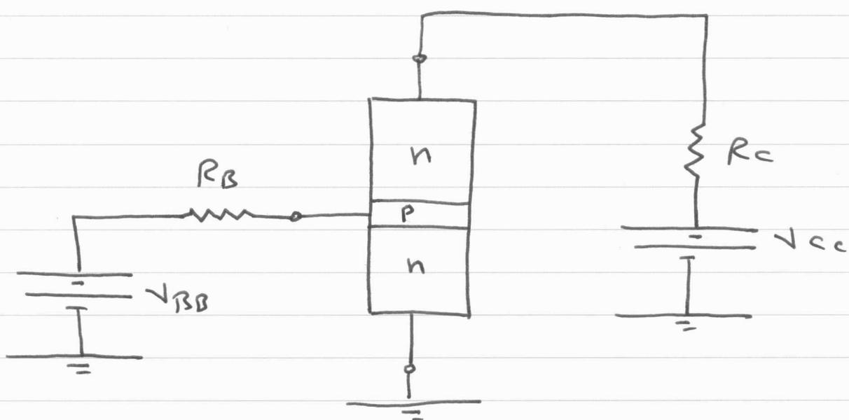
Since the base-emitter junction is forward biased; the transistor could be either in the active or the saturation region
