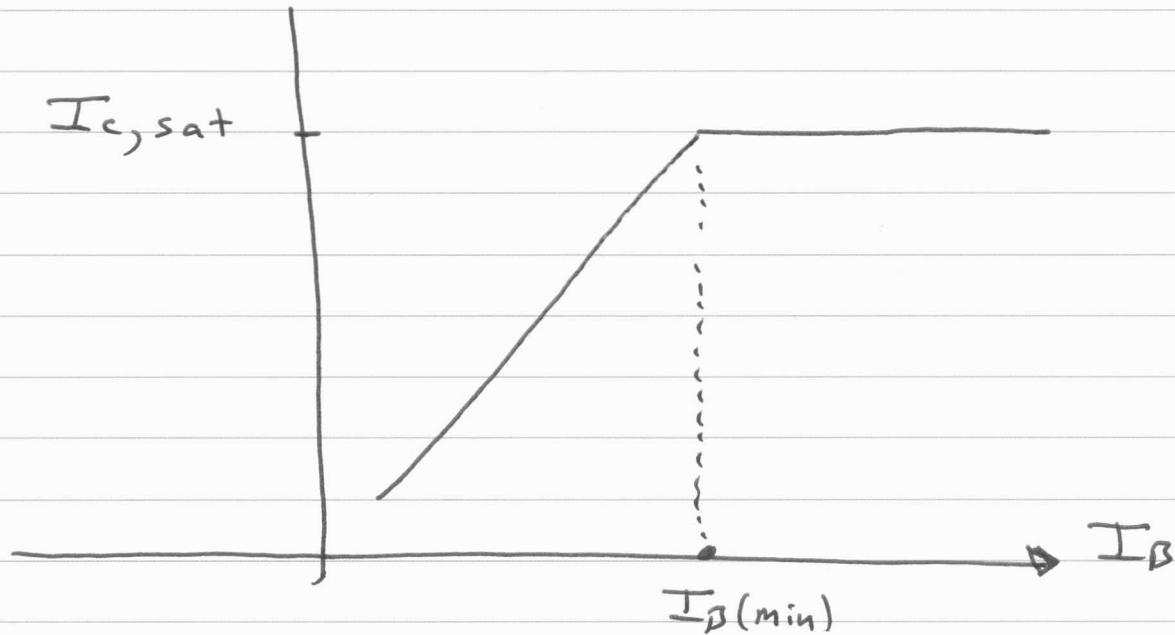
$$I_b(\min) = \frac{I_{c,sat}}{\beta}$$
