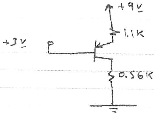
$$V_{EB} = V_E - V_B \quad \therefore V_E = 3.7 \text{ V}$$
