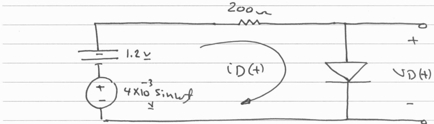
Since we have a dc source (1.2V) and an ac signal ( $4 \times 10^{-3} \sin \omega t$ ) and the diode is always on; we use Superposition theorem to find  $v_D(+)$
