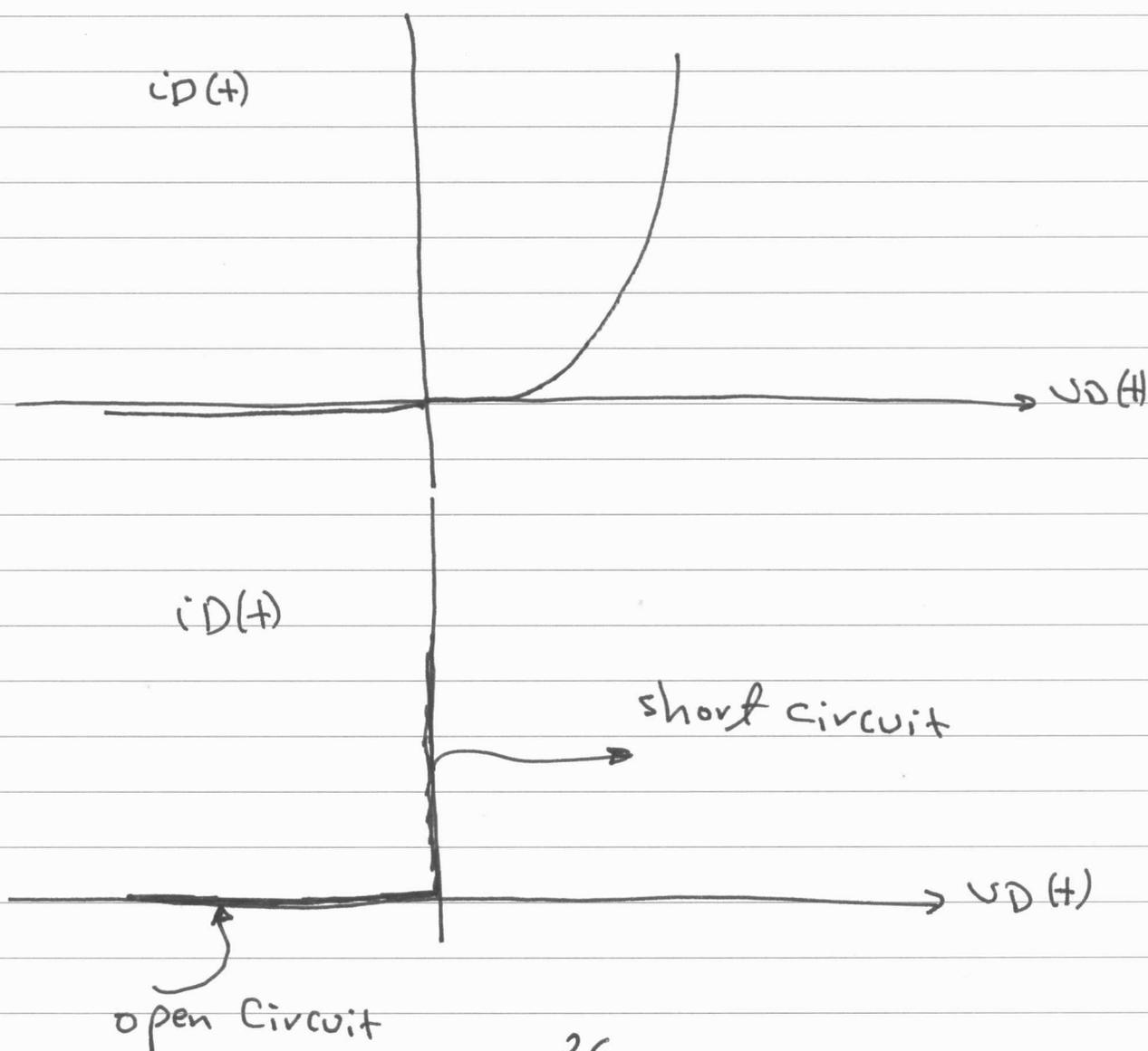
\* When  $V_s \geq 0$ ; the Diode is on, and replaced with short circuit
