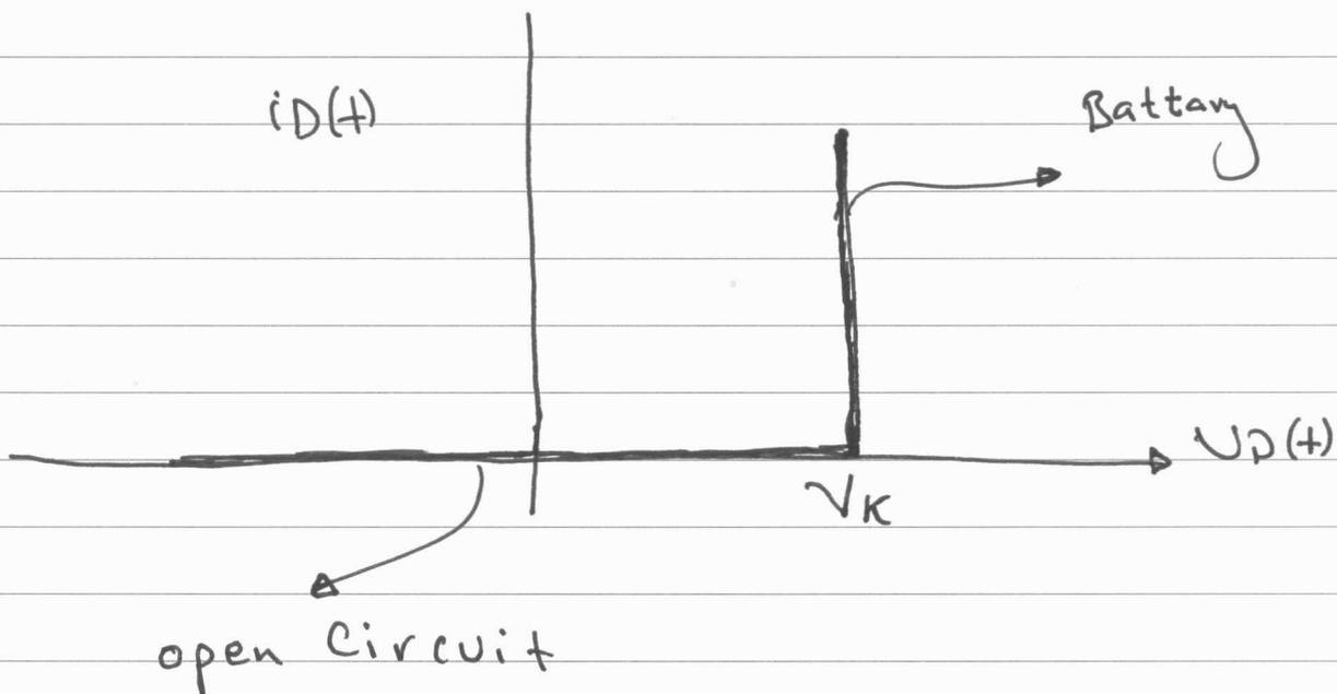
\* When  $V_s \geq V_K$ , the diode is on and replaced with a constant voltage
