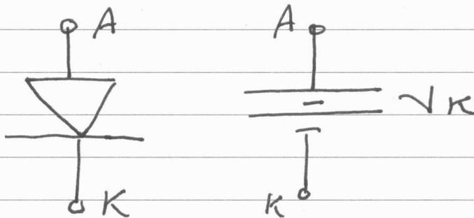
\* When  $V_s < V_K$ , the diode is off and replaced with open circuit
