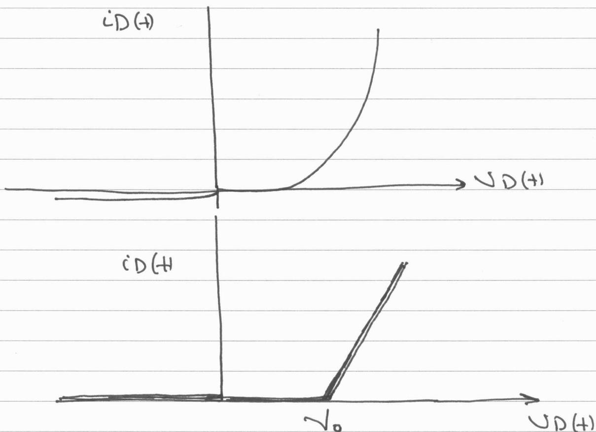
\* When  $v_s \geq V_0$ , the diode is on, and replaced with
