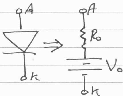
\* When  $v_s < V_0$ , the diode is off, and replaced with open circuit
