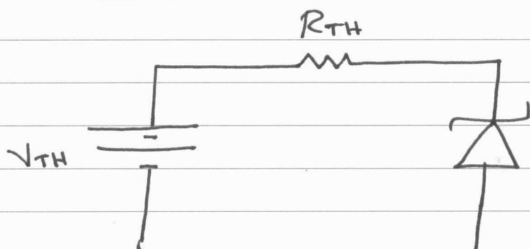
$$R_{TH} = 1\text{ k} \parallel 2\text{ k} = 0.67\text{ k}$$
