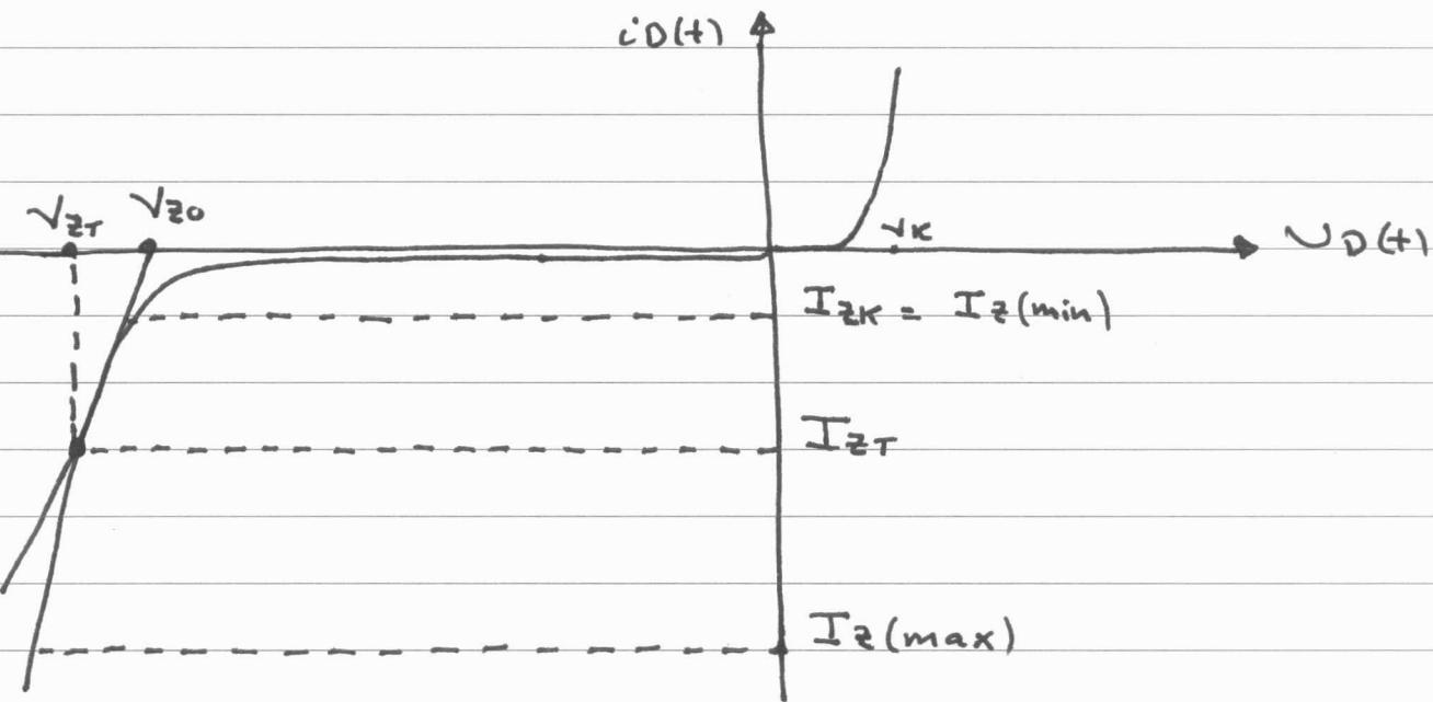
The Model of the Zener diode in the breakdown
