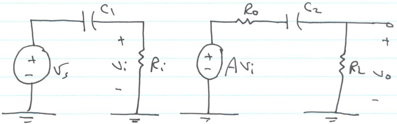
$$V_o = \frac{R_L}{R_L + R_o + \frac{1}{j\omega C_2}} A V_i$$
