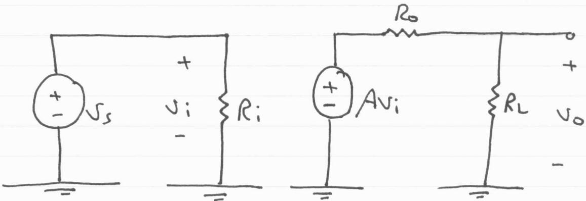
$$V_o = \frac{R_L}{R_L + R_o} A V_i$$
