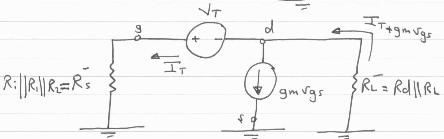
$$R_L^- (I_T + g_m V_{gs}) + R_S^- I_T = V_T$$
