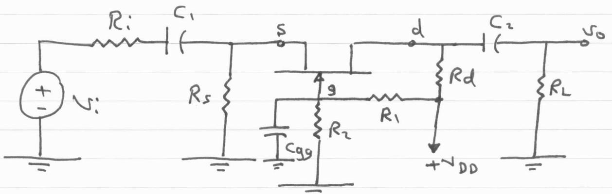
$$R_i = 0.3\text{K}, R_1 \parallel R_2 = 100\text{K}, R_d = R_L = 5\text{K}$$
