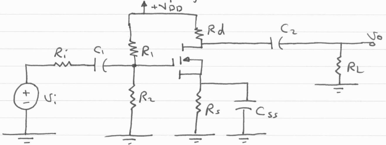
$$R_i = 0.3\text{K}, \quad R_1 \parallel R_2 = 100\text{K}, \quad R_d = R_L = 5\text{K}$$
