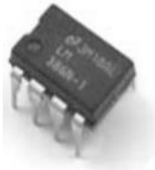
(a) Op Amp 741 8-pins DIP package
