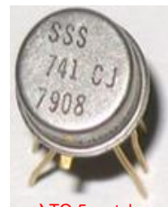
(c) TO-5 metal can 8-Leads package
