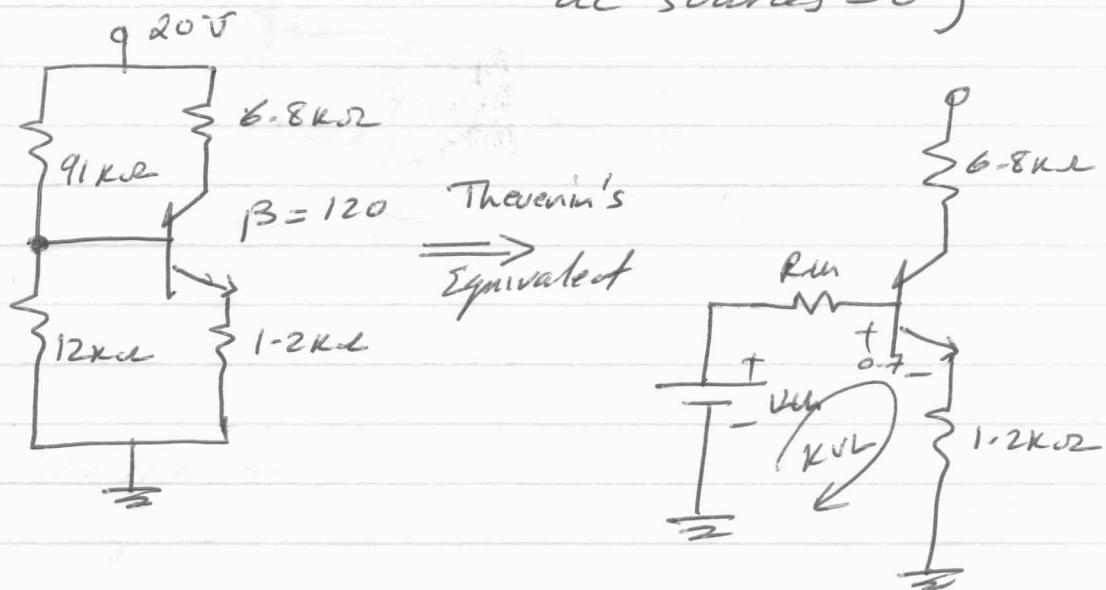
where  $V_{th} = \frac{12k\Omega}{12k\Omega + 9k\Omega} \cdot 20 = 2.33 \text{ V}$
