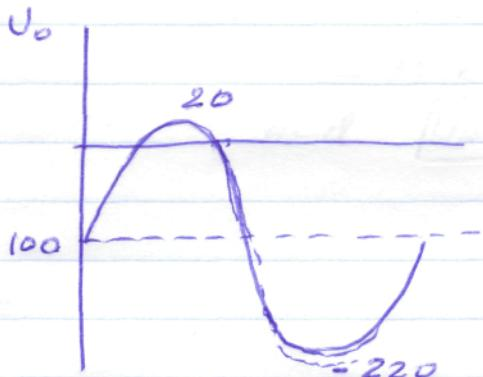
Note using an ideal diode model is a good approximation in both cases since for (a) we have 240 instead of 239.7 V & for (b) we have 20 instead of 20.7
