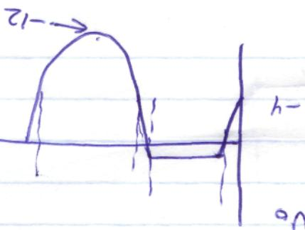
2) otherwise when  $U_i < V_D$  diode is off  $\Rightarrow U_o = U_i - V_D$
