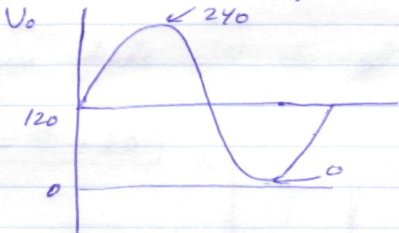
b) starting with positive  $U_i \rightarrow$  diode is ON
