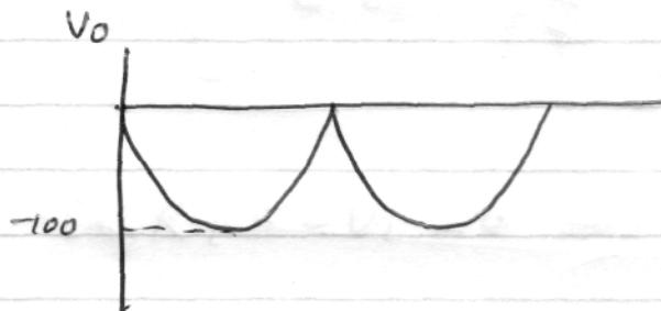
$$\text{PIV} \geq 100 \text{ V}$$
