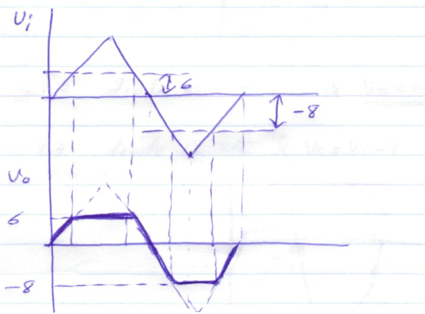
Q37. Both are clapper circuits
