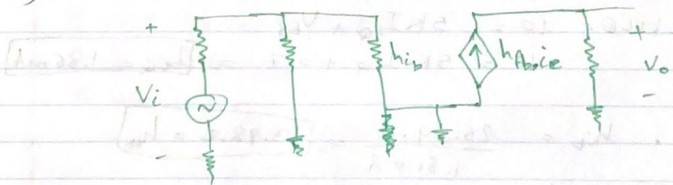
$$i_i = \frac{V_i}{Z_i + R_s} \quad \text{for } R_s = 50\Omega \quad A_v = 62.5$$
