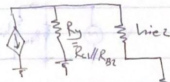
$$i_{b1} = \frac{V_i}{h_{ie1}} \quad \textcircled{1} \quad \textcircled{2} \quad \textcircled{4}$$
