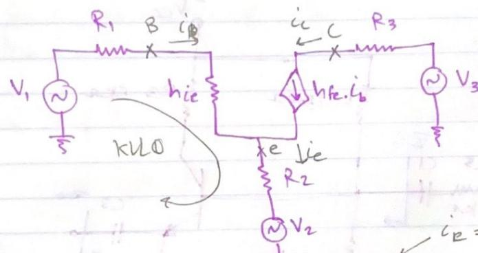
$$V_1 = R_1 i_b + h_{ie} i_b + R_2 (\beta + 1) i_b + V_2$$
