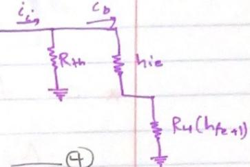
$$Z_i = R_{th} // (h_{ie} + 1k\Omega(h_{fe}+1)) \quad \textcircled{4}$$
