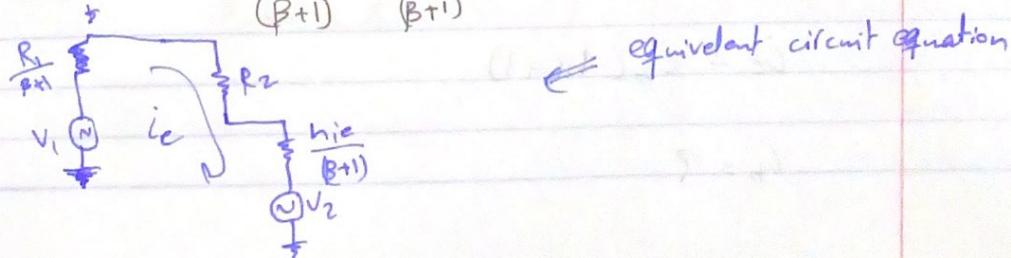
→ Collector Equivalent Circuit
