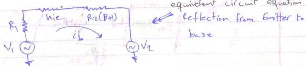
$$* i_e = \frac{V_1 - V_2}{\frac{R_1}{(\beta + 1)} + \frac{h_{ie}}{(\beta + 1)} + R_2} \leftarrow \text{emitter loop}$$
