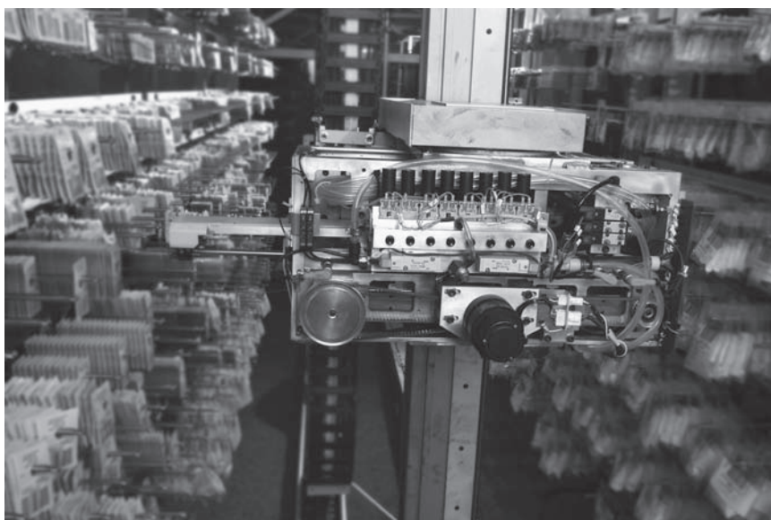
FIGURE 12.1 A robot in a hospital pharmacy selects medications by bar code
