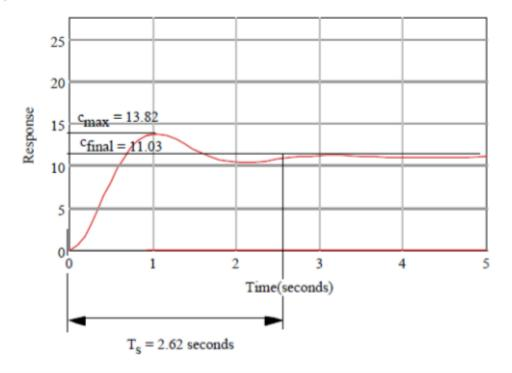
and  $T_s = 2.62$  seconds. Estimating a second-order system, we use Eq. (4.39) to find  $\zeta = 0.4$ , and Eq. (4.42) to find  $\omega_n = 3.82$ . Thus,  $G(s) = \frac{K}{s^2 + 2\zeta \omega_n s + \omega_n^2}$ . Since  $C_{\text{final}} = 11.03$ ,  $\frac{K}{\omega_n^2} = 11.03$ . Hence,
